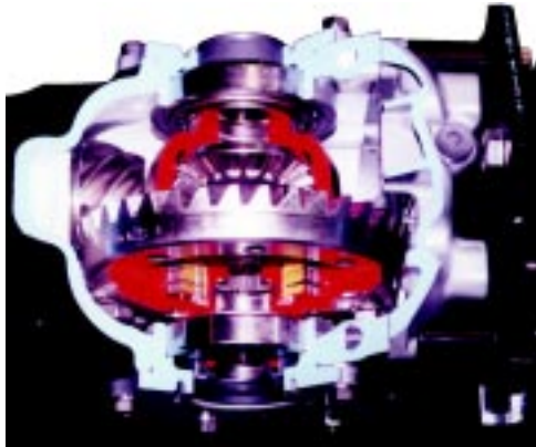
Subaru differential with very clever limited slip clutch assembly (highlighted in yellow).
